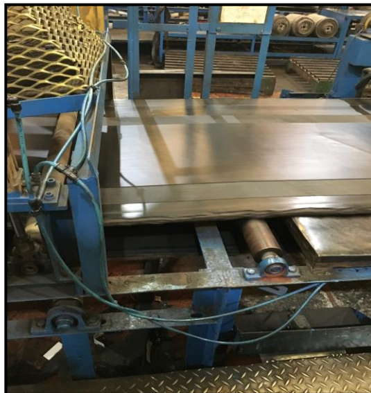
Gambar 4.5 Proses Pelapisan Ply ( Squeegee ) (Sumber : PT XYZ, 2019)
