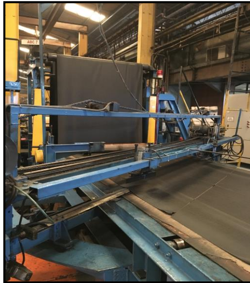
Gambar 4.4 Proses Pemotongan Treatment ( Bias Cutting ) (Sumber : PT XYZ, 2019)
