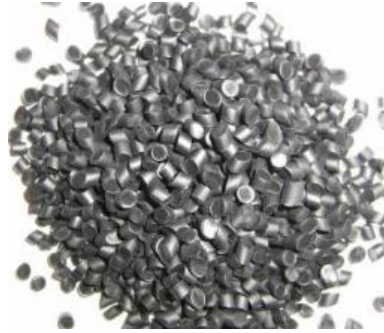
Gambar 2. EPDM (Ethylene Propylene Diene Monomer )
