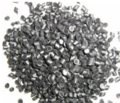
Gambar 8. EPDM (Ethylene Propylene Diene Monomer )
